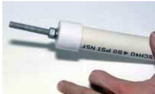
Figure 8e. Install the end cap foot onto the bottom section of the PVC pole.
