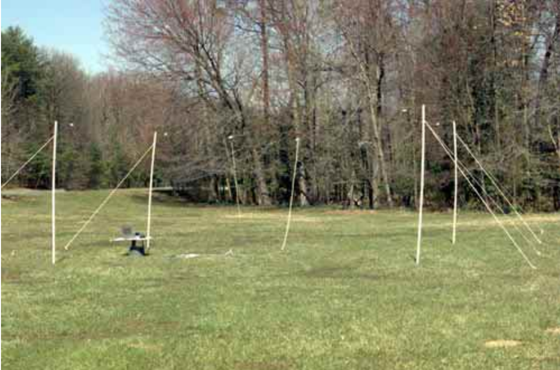
Figure 10m. Completed JOVE receiver and antenna setup.
