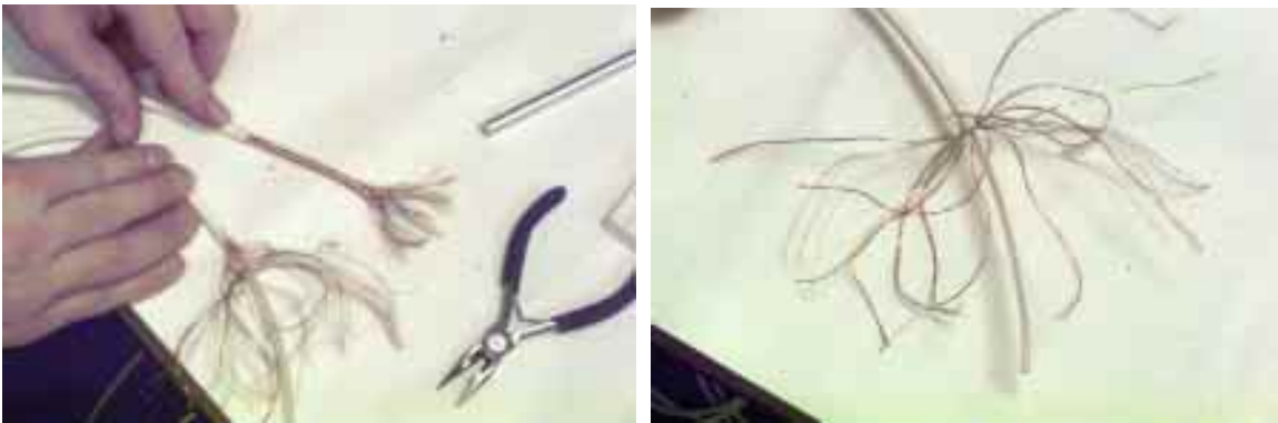
Figure 3a and 3b. Unbraid the copper shielding.
